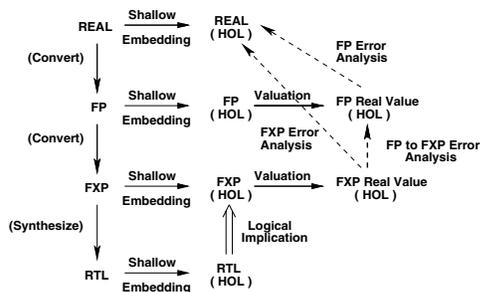
Fig. 2. DSP Specification and Verification Approach [1]
