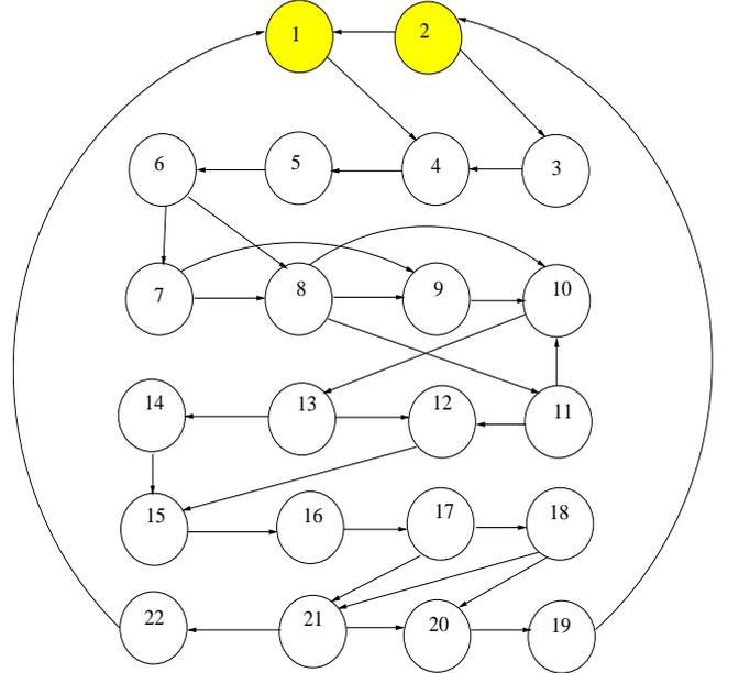
Fig. 4. ASTG of Region  $R_1$  for the Circuit in Figure 2
