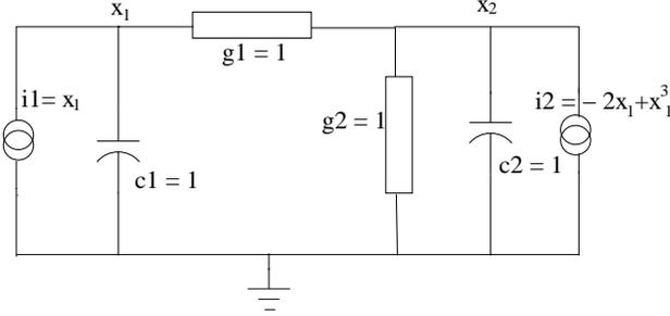
Fig. 2. Oscillating Circuit Example
