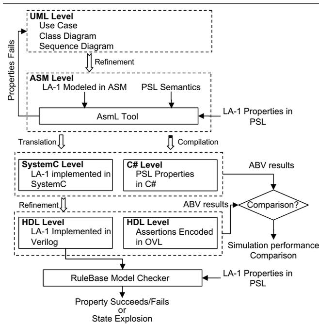
**Figure 2. Look-Aside Interface Design and Verification Methodology.**
