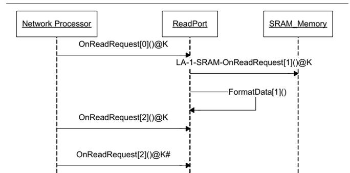
**Figure 3. Sequence Diagram for the Reading Mode.**
