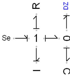
**Fig. 9.** Tunnel Diode Causal Simplified Bond Graph
