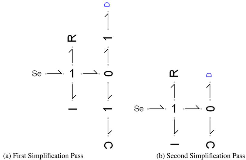
**Fig. 8.** Tunnel Diode Bond Graph Simplifications
