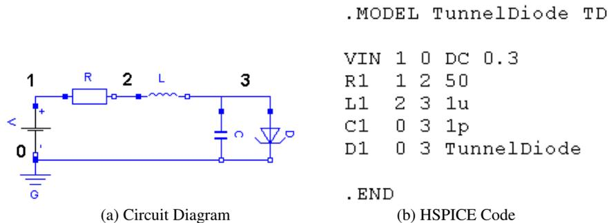
Fig. 5. Tunnel Diode Oscillator
