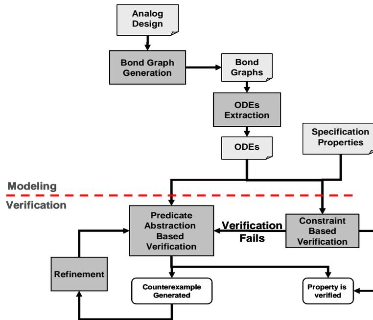
Fig. 1. Proposed Verification Flow
