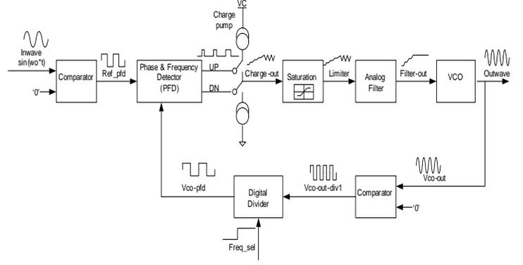
Fig. 3. PLL Frequency synthesizer diagram
