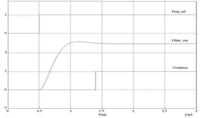
Fig. 4. PLL Frequency Synthesizer Run-Time Simulation
