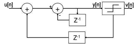
Fig. 2. First-order  $\Delta\Sigma$  Modulator
