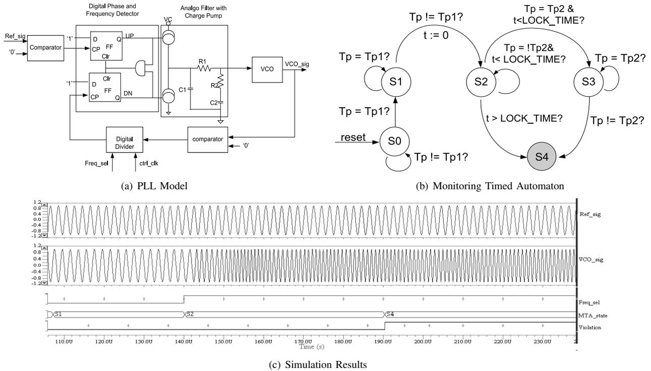
Fig. 3. Frequency Synthesizer
