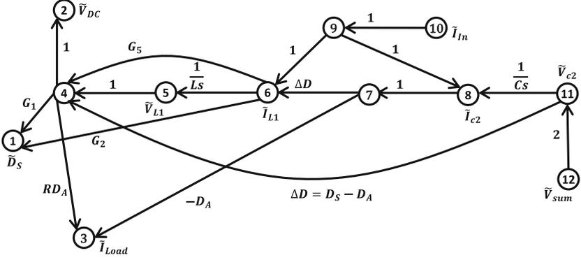
Fig. 4. Signal flow graph of Z-source converter transpose
