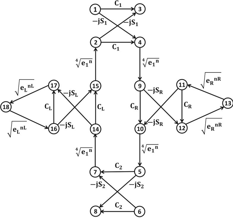
Fig. 6. Signal flow graph of the PANDA resonator
