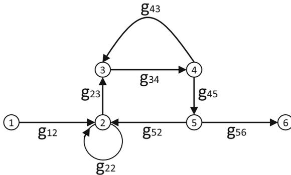
Fig. 1. A signal-flow graph
