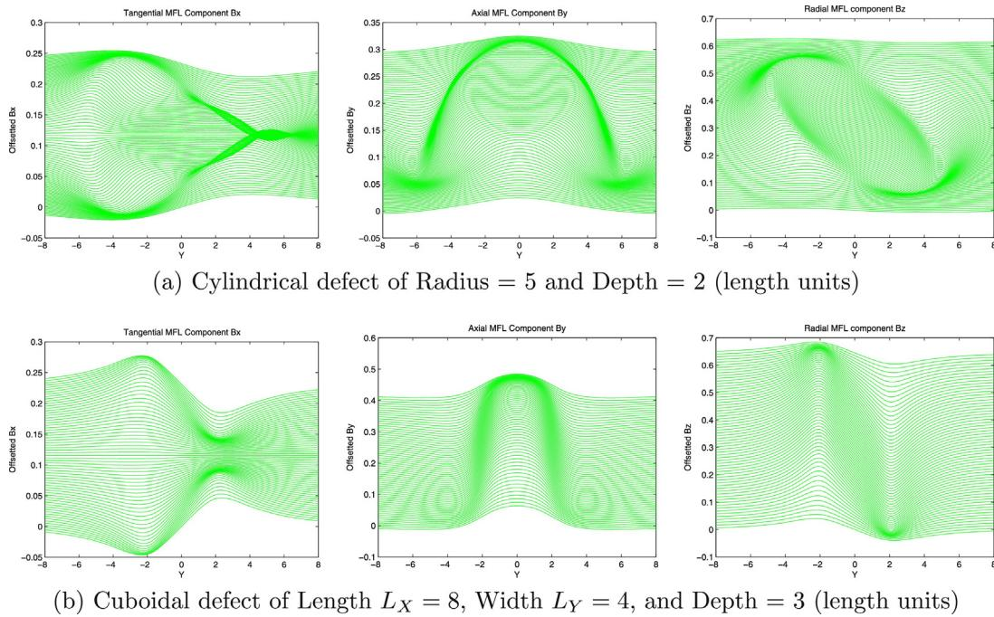
**Fig. 5.** MFL signals from each of the sensors passing above a defect.
