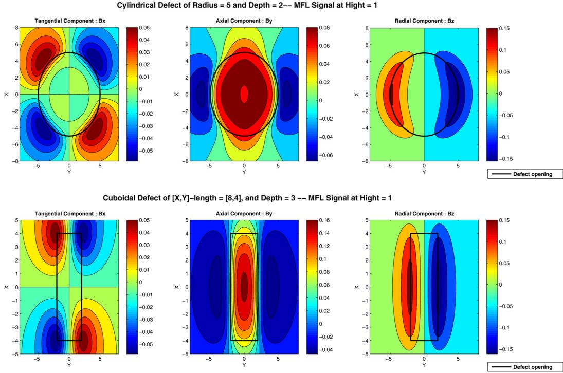
**Fig. 4.** MFL scan of cylindrical (top) and cuboidal (bottom) defects.
