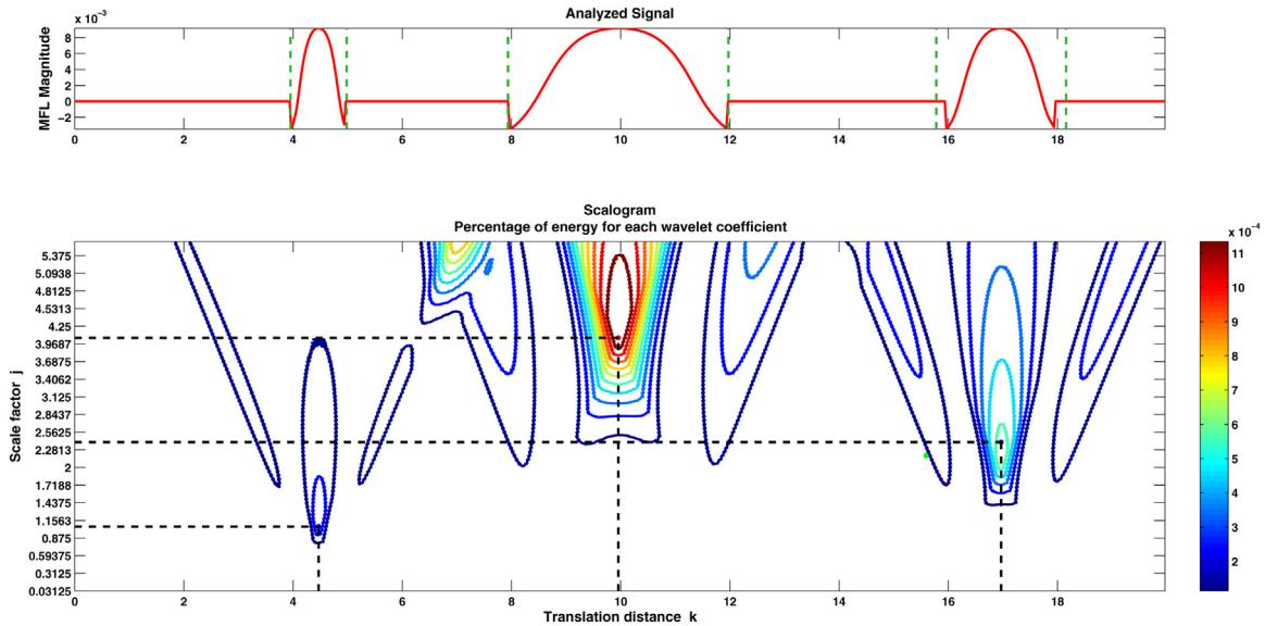
**Fig. 8.** Wavelet transform of an MFL signal with respect to a pattern-adapted wavelet basis.
