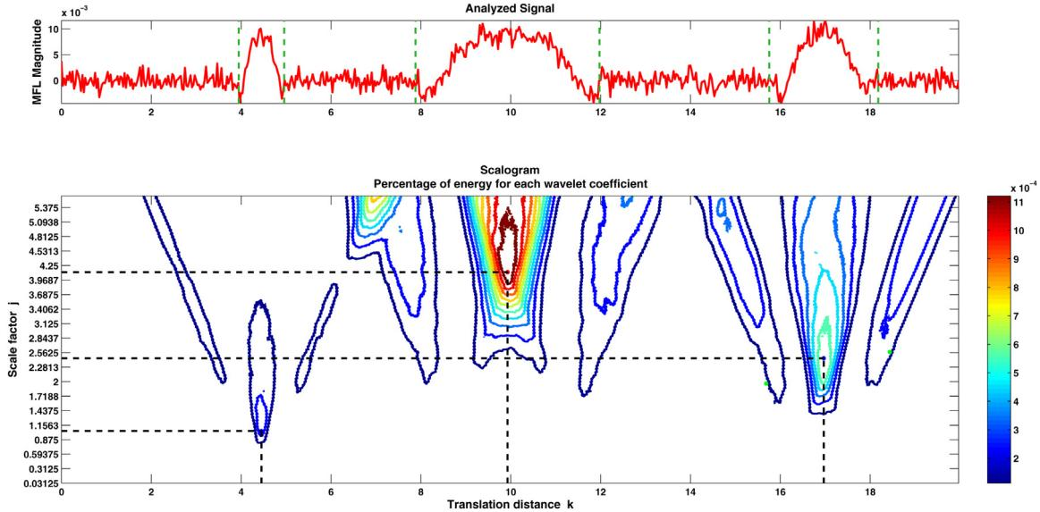
**Fig. 10.** Defect detection in MFL signal with White Gaussian Noise (SNR = 10 dB).
