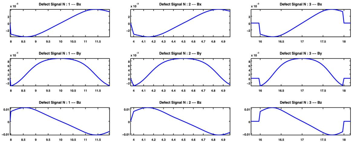
**Fig. 9.** Portions of the MFL signal in Fig. 8 corresponding to metal-loss defects.
