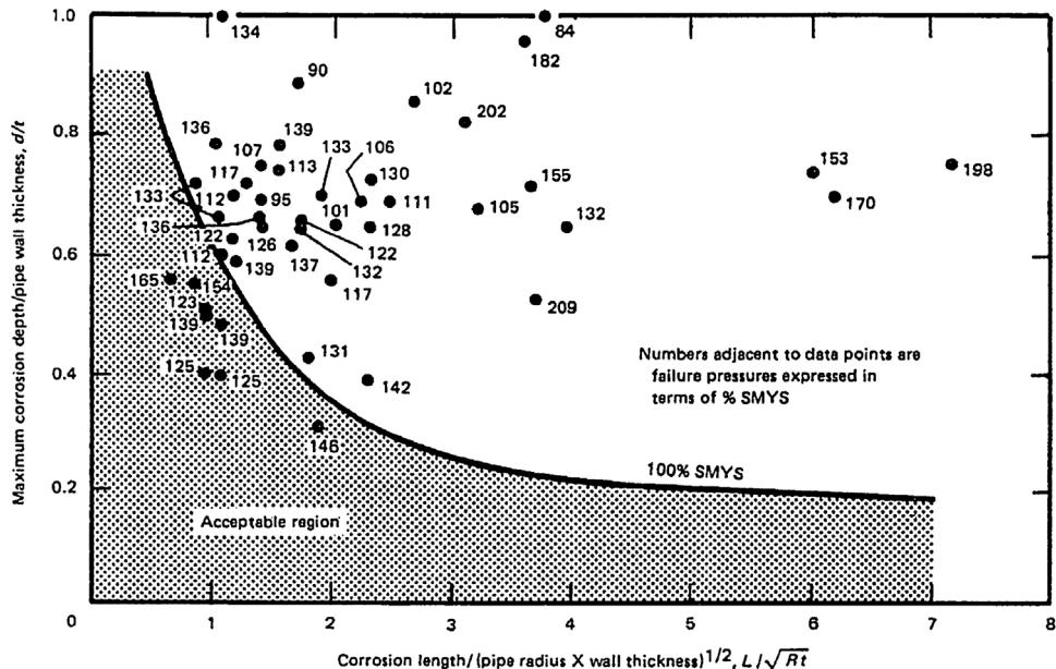
**Fig. 12.** Parabolic criteria for classifying corrosion defects based on length and depth, for a given pipeline material and operating pressure [3].
