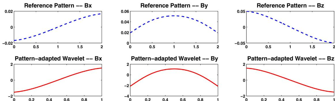
**Fig. 7.** Reference patterns and admissible mother wavelets for defects of cuboidal shape.
