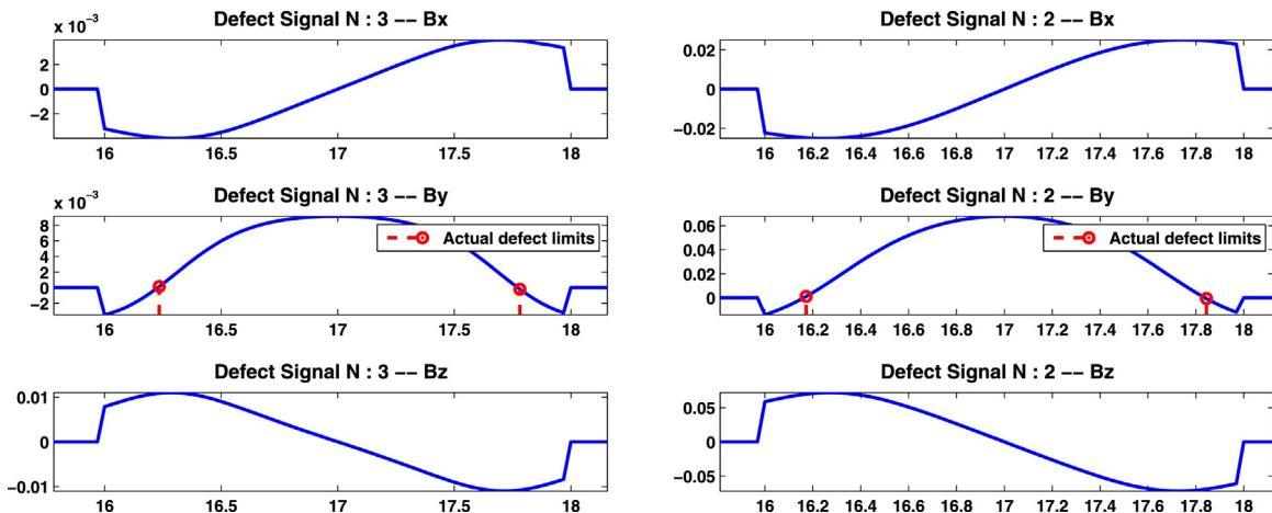
**Fig. 13.** Difference in MFL magnitude for cylindrical defects of same radius and different depths.
