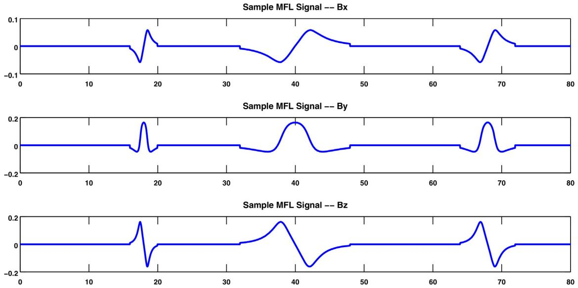
**Fig. 6.** Sample MFL scan of a pipeline with three metal-loss defects of cuboidal shape.
