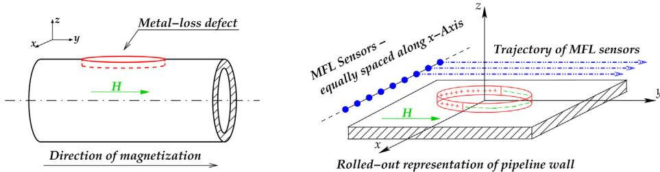
Fig. 3. MFL measurement setting.
