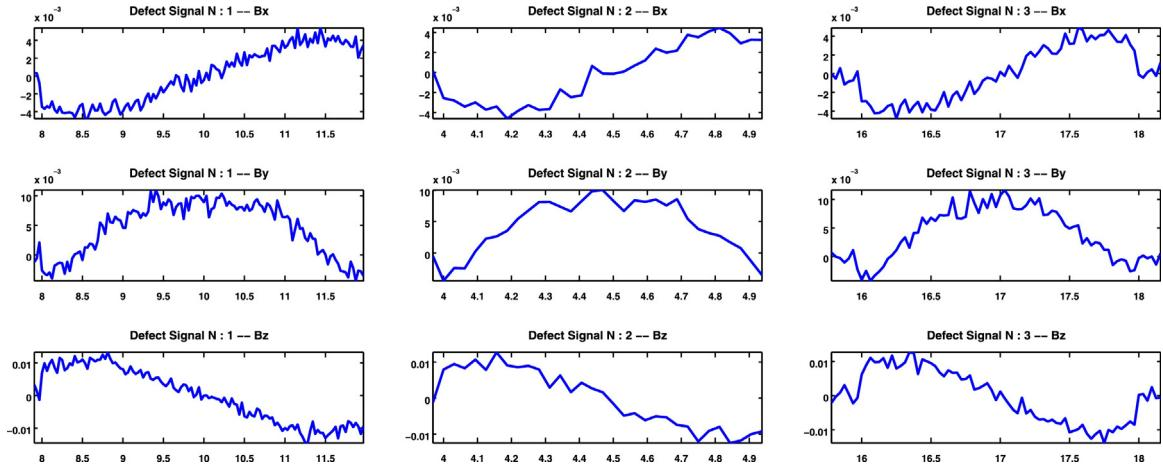
**Fig. 11.** Portions of the MFL signal in Fig. 10 corresponding to metal-loss defects.
