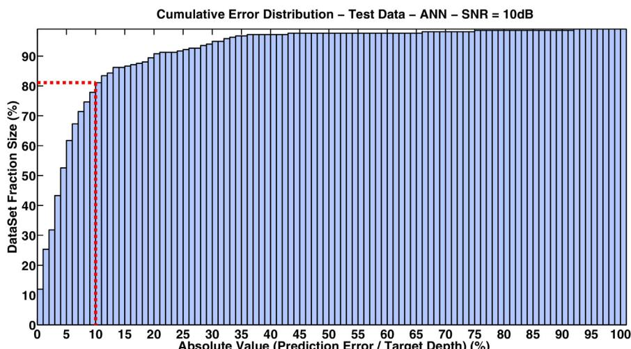
Fig. 16. Depth prediction accuracy of 2-layer ANN – SNR = 10 dB (The dotted lines indicates the accuracy @80%).
