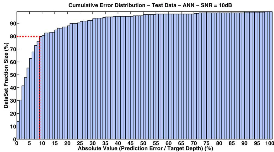
**Fig. 17.** Depth prediction accuracy of 3-layer ANN – SNR = 10 dB (The dotted lines indicates the accuracy @80%).
