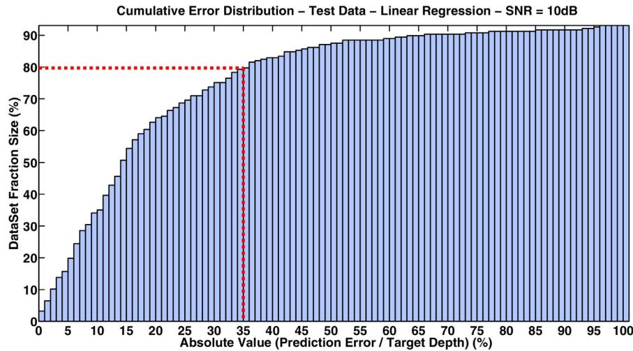
**Fig. 18.** Depth prediction accuracy of linear regression – SNR = 10 dB (The dotted lines indicates the accuracy @80%).
