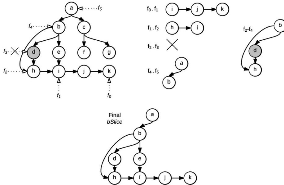
Figure 10. Steps of Algorithm 1 where  $f_3$  is corrupted.
