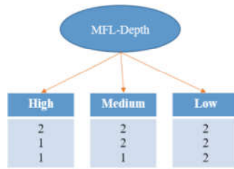
Fig. 6. The decision tree for the MFL-depth attribute. The defect status of type I is referred to by 1; while type II is referred to by 2.
