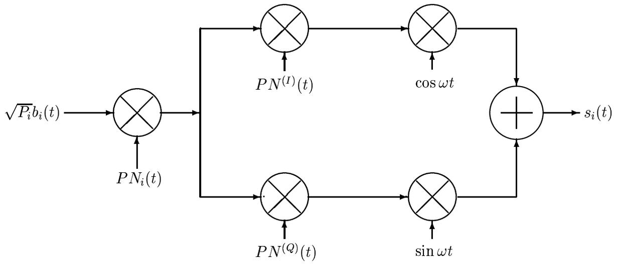
Figure 1: Transmitter model for the  $i$ -th user
