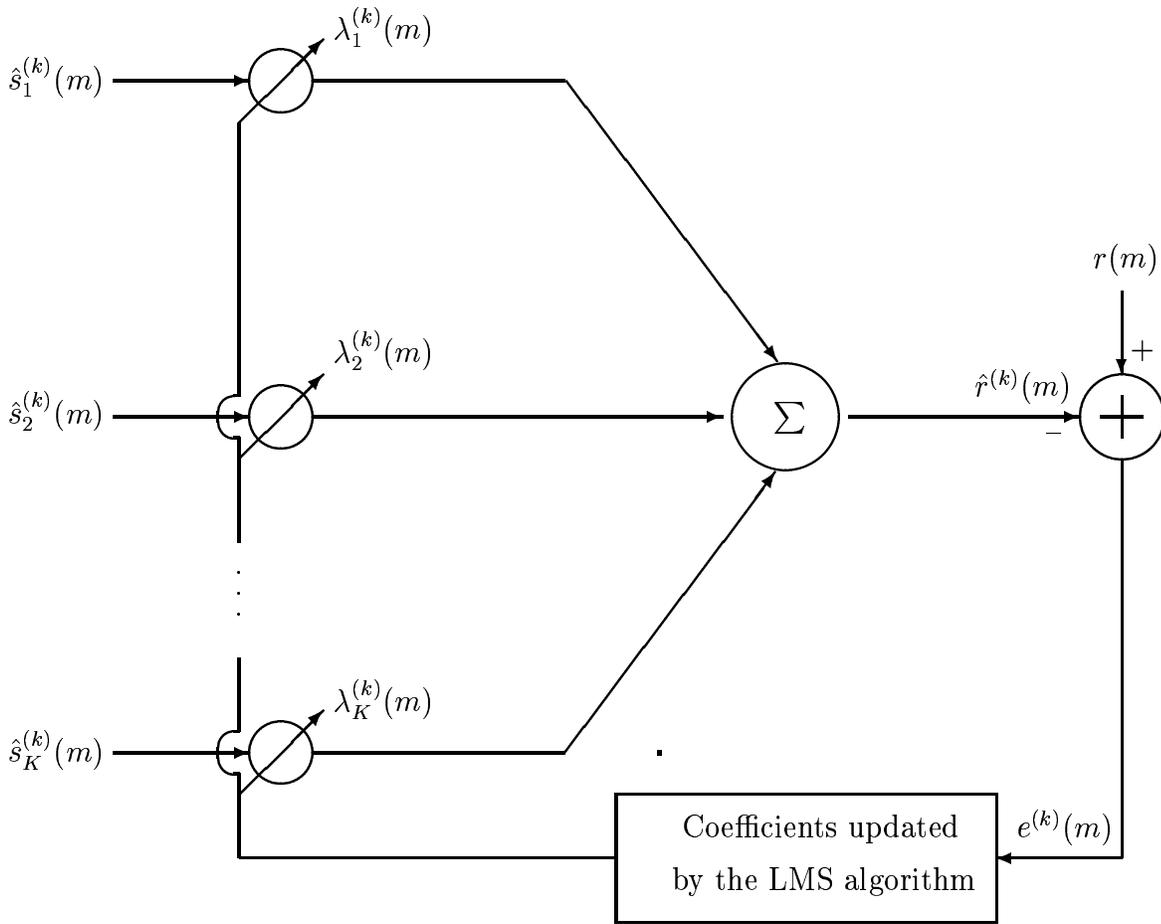
Figure 3: Weight updating in the adaptive multistage PIC in the AWGN channel
