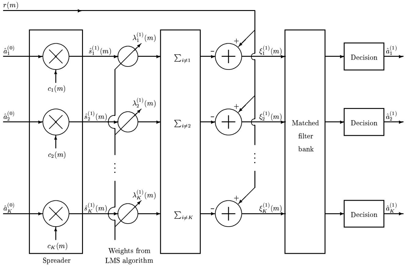
Figure 2: One stage of the adaptive multistage PIC detector in the AWGN channel
