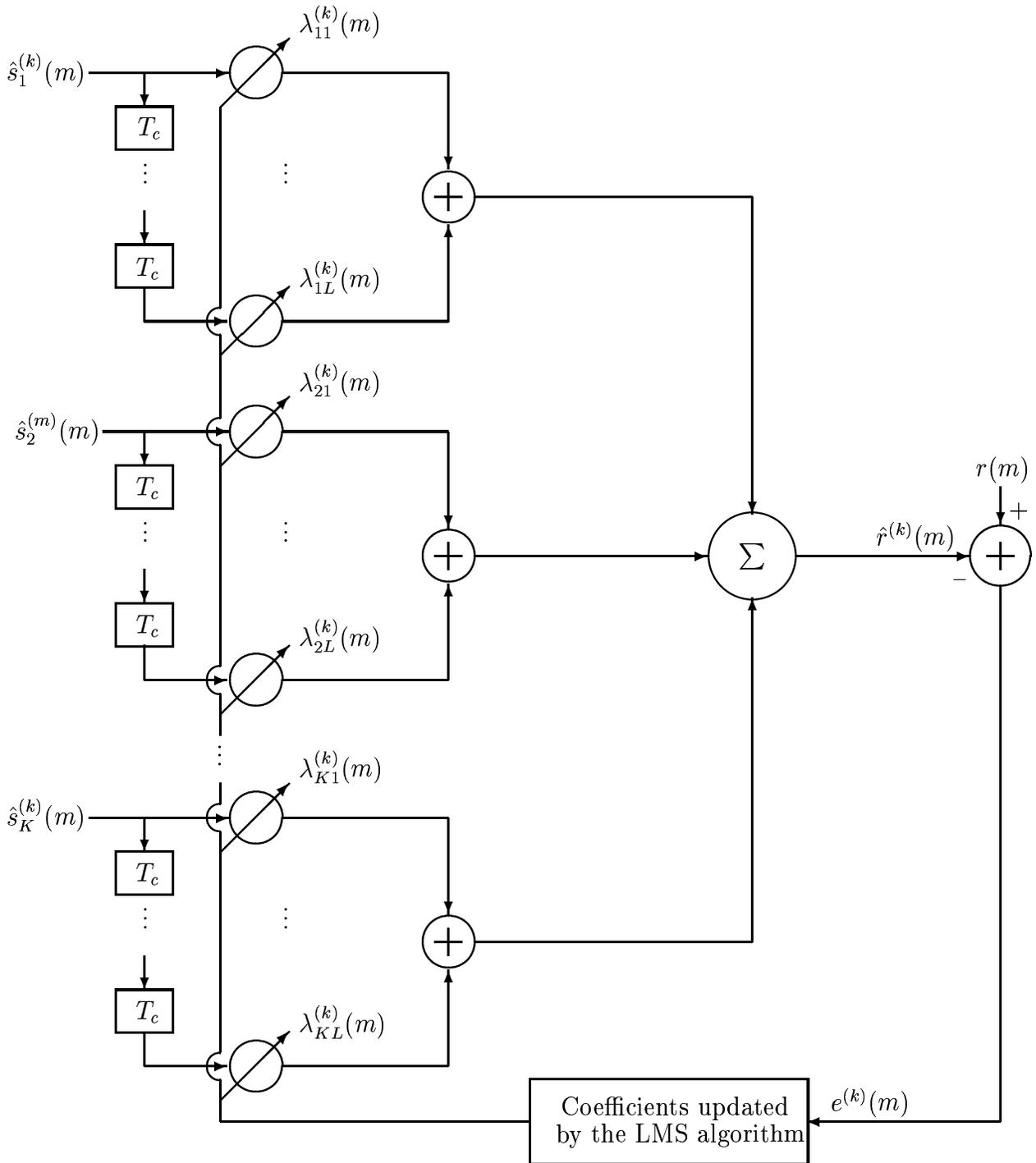
Figure 4: Weight updating in the adaptive multistage PIC in a multipath fading channel
