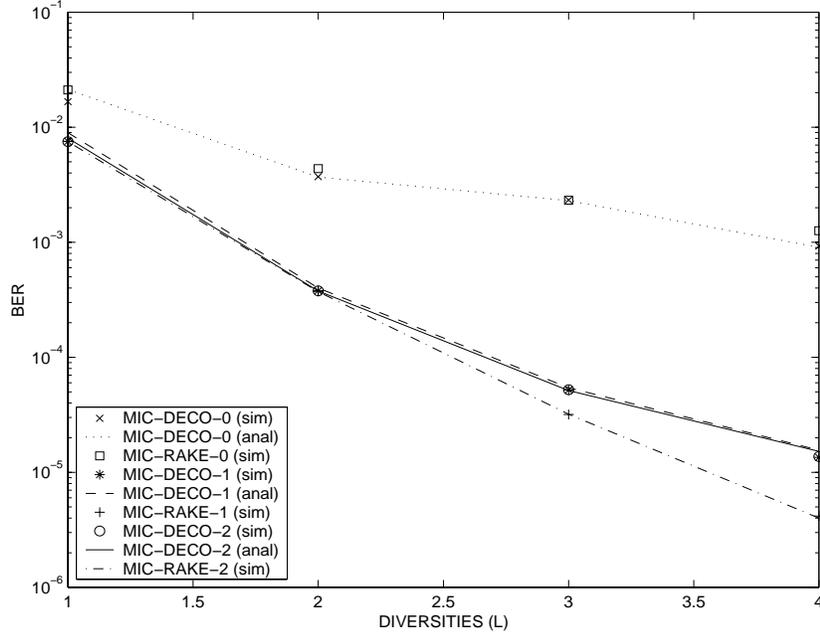
Fig. 3: BERs of the MIC-DECO and MIC-RAKE in a 3-user system over L-path ( $L=1,2,3,4$ ) Rayleigh fading channels. (SNR=20dB,  $N=31$ , equal-power users. Imperfect channel knowledge,  $\sigma_e^2 = 10^{-2}$ .)
