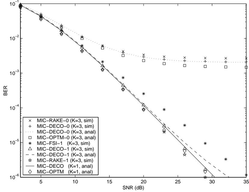
Fig. 1: BERs of the MIC schemes in a 3-user system over a 2-path Rayleigh fading channel. ( $N=31$ , equal-power users. Perfect channel knowledge).
