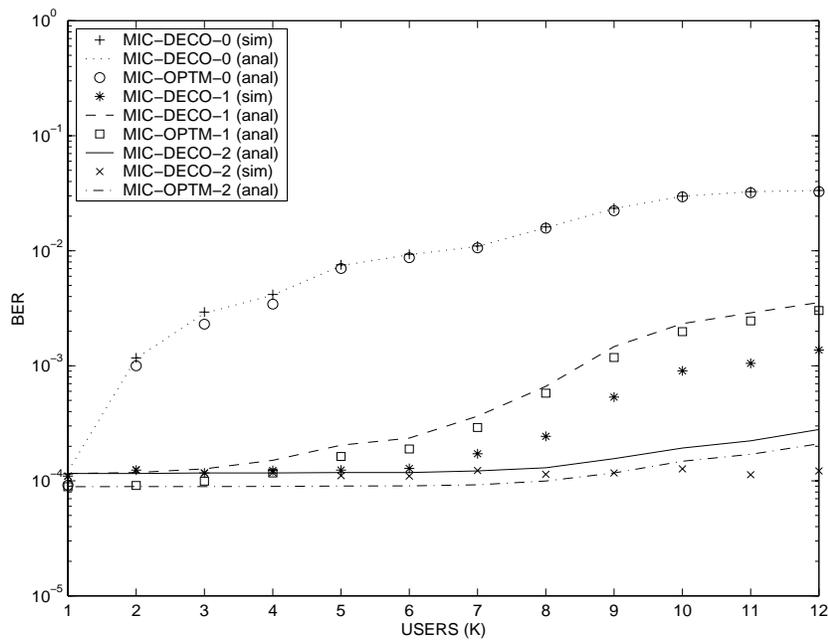
Fig. 2: BERs of the MIC-DECO and MIC-OPTM in a multi-user system over a 2-path Rayleigh fading channel. (SNR=20dB,  $N=31$ , equal-power users. Perfect channel knowledge).
