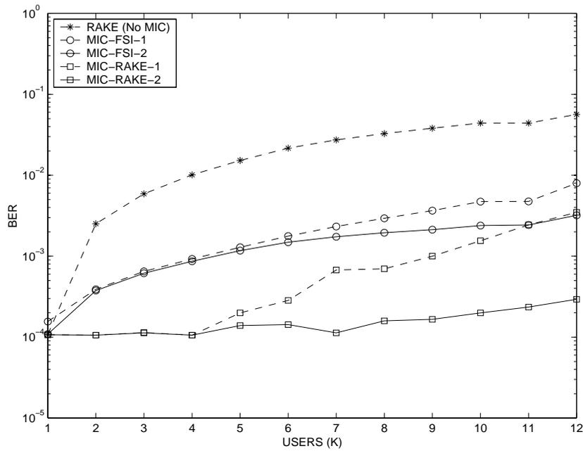
Fig. 4: Simulation results on the BER of the MIC-FSI and MIC-RAKE in a multiuser system over a 2-path Rayleigh fading channel. (SNR=20dB,  $N=31$ , perfect channel knowledge, long PN sequence.)
