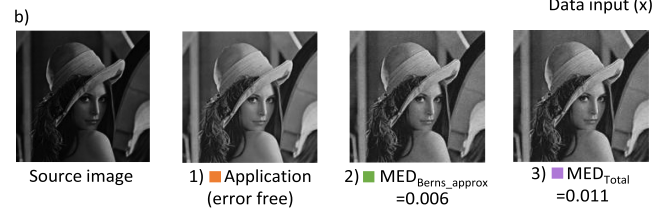
FIGURE 8. Gamma correction application: a) Output pixels according to input pixels in the range [0, 1] for 1) \Upsilon = 0.45 , 2) 4 th order polynomial function, and 3) simulation results for n = 4 , BSL = 1024 , and BER = 10^{-1} . b) The corresponding results for processing a 160 \times 160 image.
